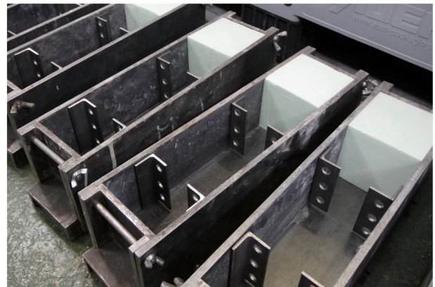
Fig. 4. Steel mold equipped with sacrificed L-shaped profiles for creep and shrinkage prismatic specimens.
