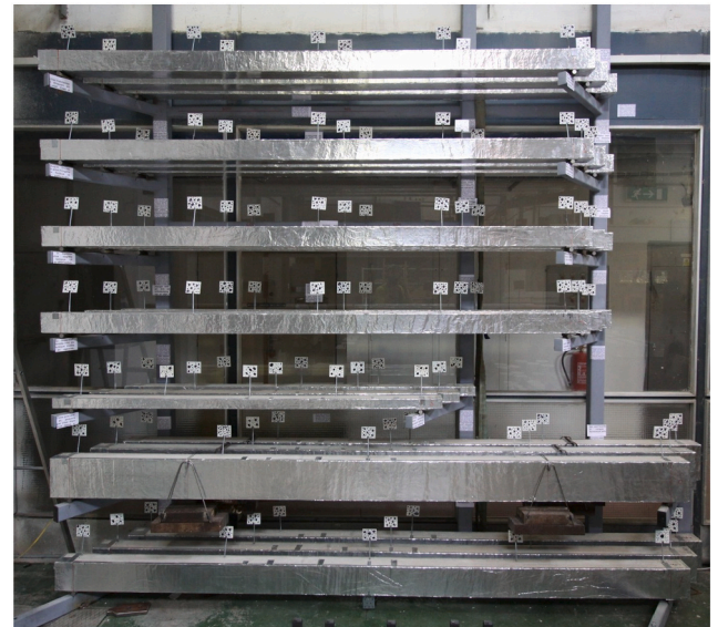
Fig. 7. Set of 7 \times 3 beams (Group I) with permanent loading, minimum span 1.75 m and maximum span 3.0 m.
