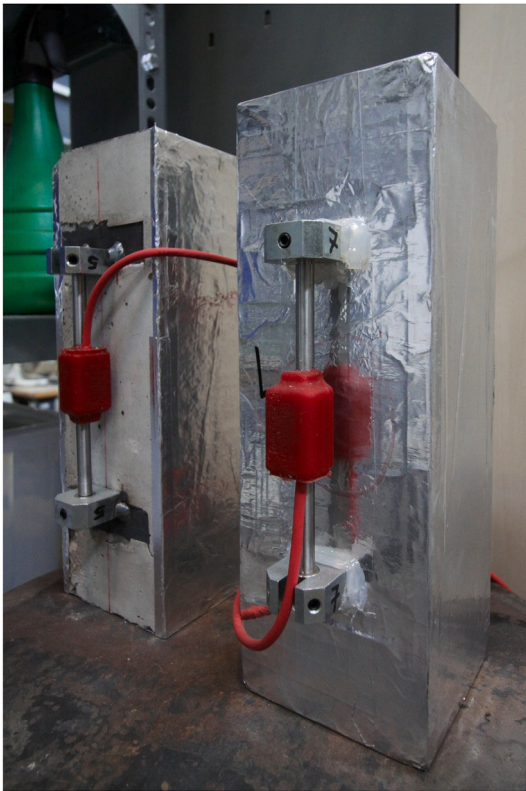
Fig. 5. Companion prismatic specimens with externally mounted VWSG for total (left) and autogenous (right) shrinkage assessment.
