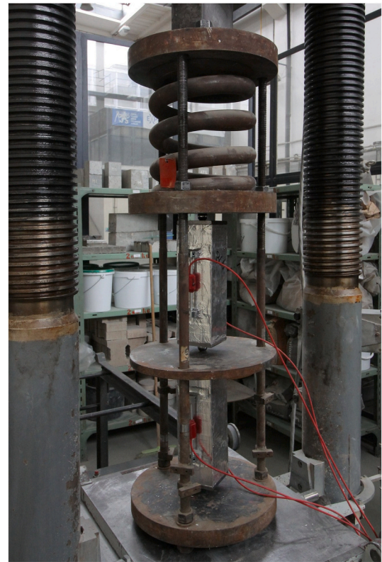
Fig. 6. Creep rig during loading.
